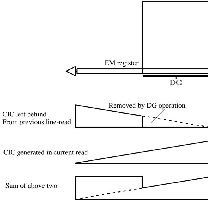
Figure 5. Explanation for how a gradient in the CIC can be induced by use of the DG.
