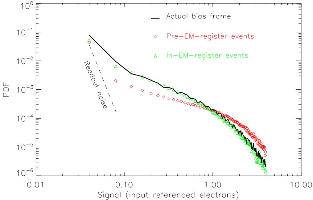
Figure 7. Model of the CIC generated both before and within in the EM register.
