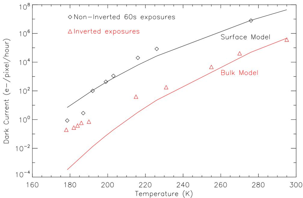
Figure 4. Comparison of dark current with manufacturers models
