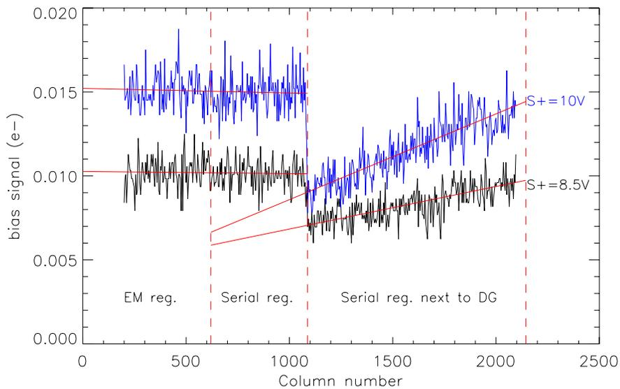
Figure 6. Actual cuts through bias frames at two values for the serial clock-hi voltage.
