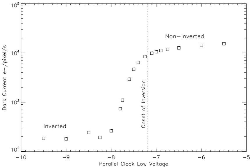
Figure 2. Measurement of the inversion point
